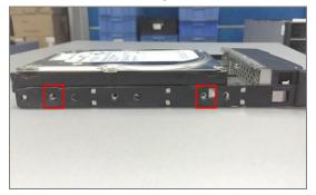
Figure 2.5 HDD Position
