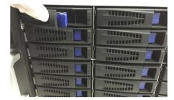
Figure 2. 7 Push the HDD Dummy into Slot
